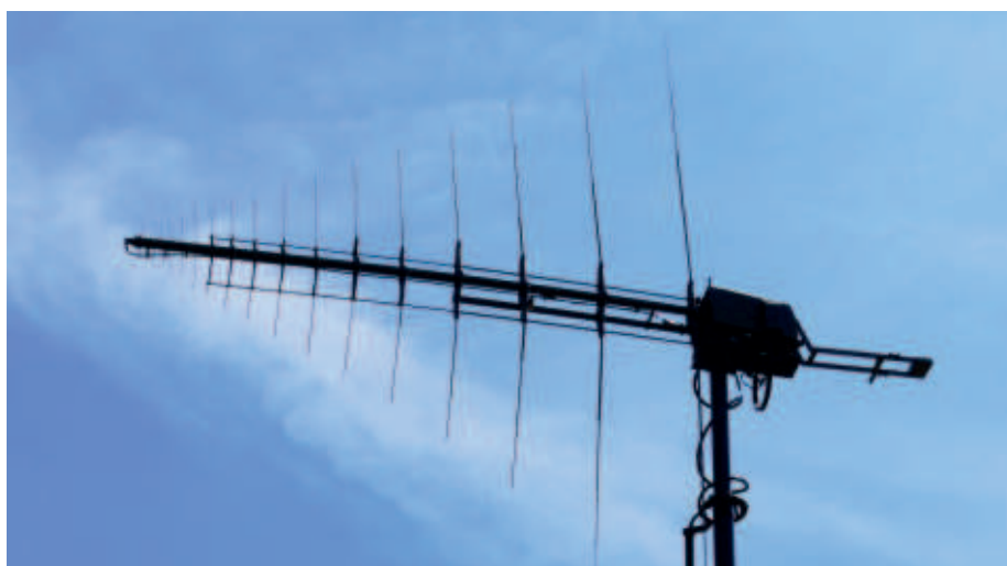
The LPDA directional broadband antenna
