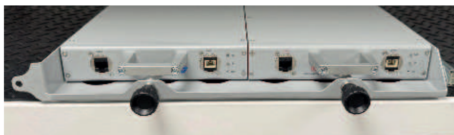
Data Diode 3D-1000 in 19" Rack Version
