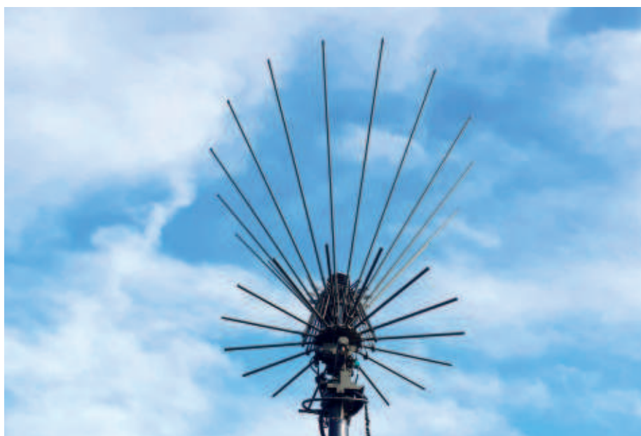
Discone omnidirectional broadband antenna
