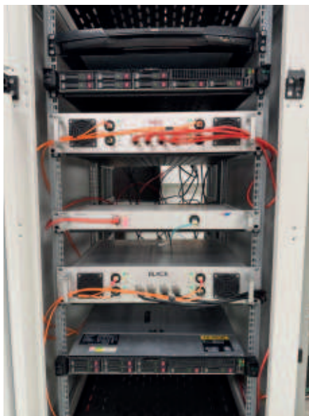
The Data Diode 3D-1000.4 in a 19" Rack version with a 3S feedback channel.
