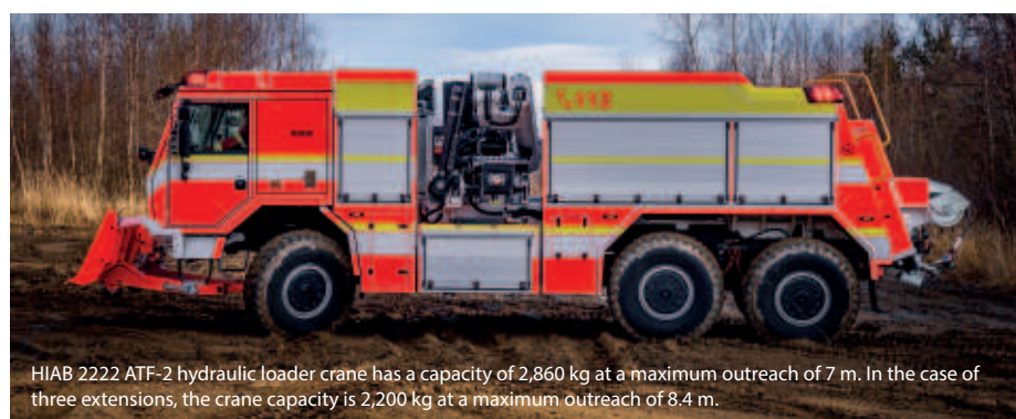
HIAB 2222 ATF-2 hydraulic loader crane has a capacity of 2,860 kg at a maximum outreach of 7 m. In the case of three extensions, the crane capacity is 2,200 kg at a maximum outreach of 8.4 m.
