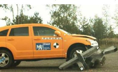
of a high-performance ballistic composite, the barriers are able to withstand commonly used small arms up to class FB 7, according to European standard EN 1522/1523. The second system, called Hystrix, was developed to slow down or stop a moving vehicle. This kind of attack has recently intensified and not only the countries directly affected have made considerable efforts to develop appropriate countermeasu-
