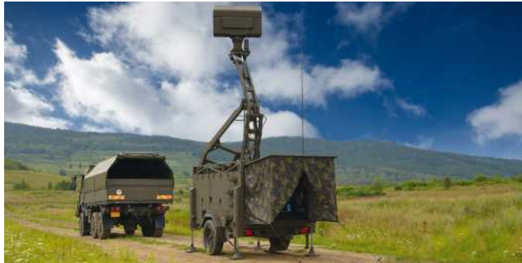
ReVISOR - complex system composed of short range radar and command and control system.
