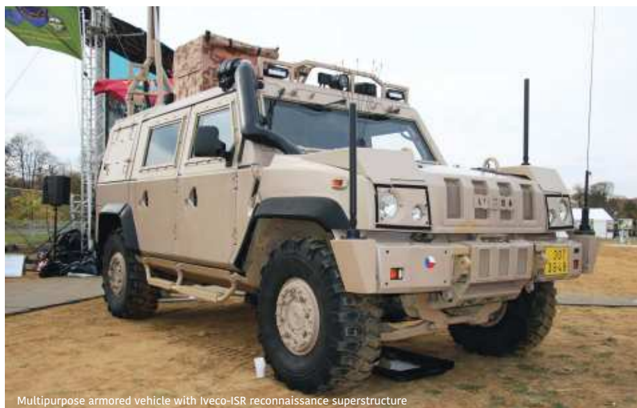
Multipurpose armored vehicle with Iveco-ISR reconnaissance superstructure
