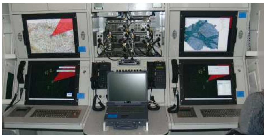
RACCOS - command and control system processes air picture data, the distribution of targets and the impact on individual targets.
