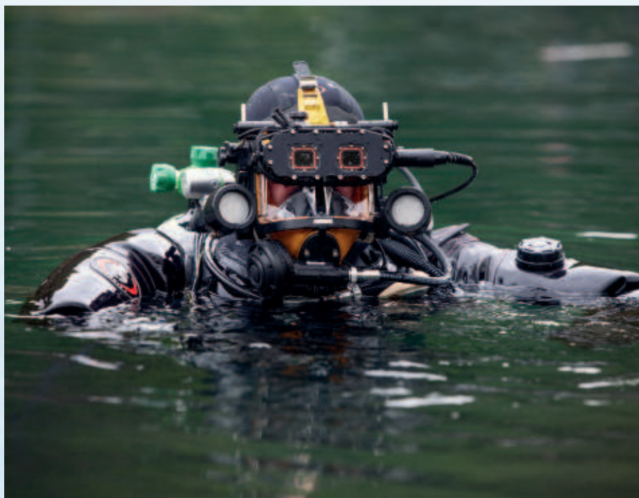
Diver with full face mask and infrared device used for seeing in invisible water
