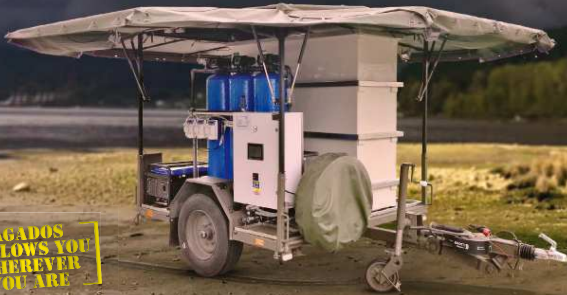
Water trailer water treatment plant
