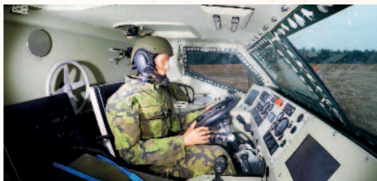
Anthropomorphic test device (instrumented dummy) in vehicle before explosion test
