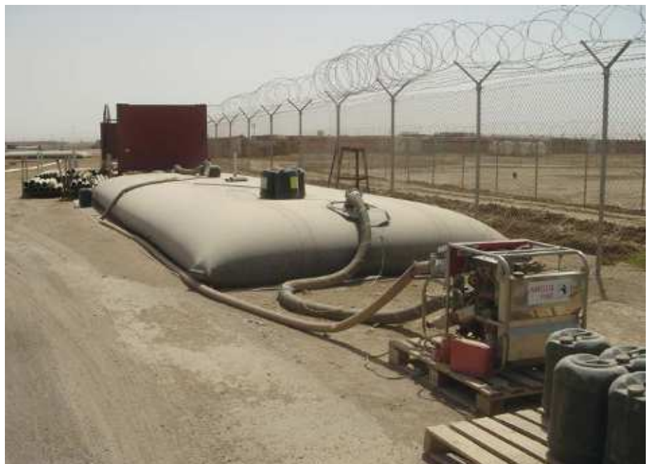
Large capacity fuel tank of up to 800,000 l volume
