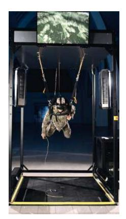
the experience of wind which is created by application of four wind modules, or the improved body tracking which allows tracking of hand movement to steer during the free fall phase more precisely. With the mounted Touch monitor, the instructor can change various exercise parameters during the running training.
