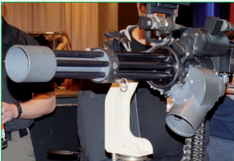
The displayed Dillon M134D Gatling Gun was pintle mounted on the Naval Post Mount and it had a magazine that holds three thousand rounds
