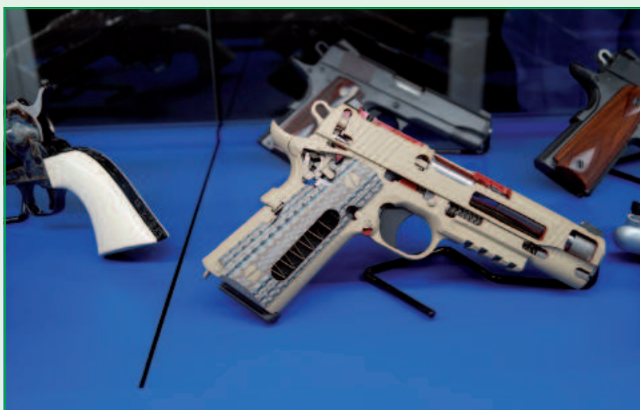
USMC soldiers' new service pistol Colt M1911A1 (cut through)
