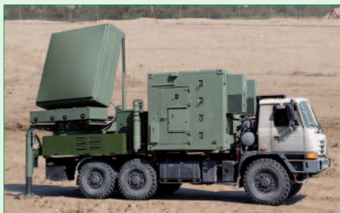
Radar společnosti IAI ELTA vyvíjený ve spolupráci s českou firmou RETIA na podvozku Tatra 6x6 IAI ELTA's radar developed in cooperation with the Czech company Retia and mounted on a Tatra 6x6 chassis
